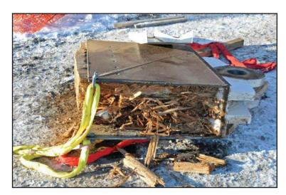
A removed section of the base shows the extent of the rotting.
